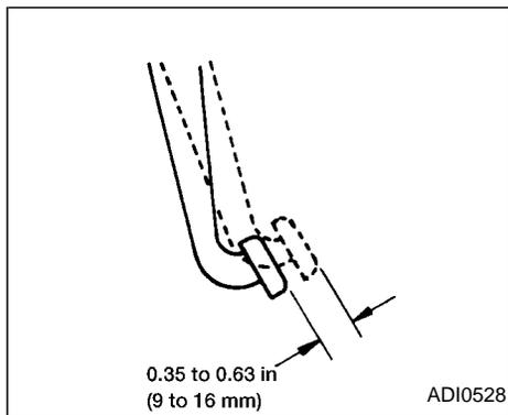
Press the pedal by hand and be sure the free travel is within the above limit. If free travel is out of the range shown above, see an authorized NISSAN dealer.
