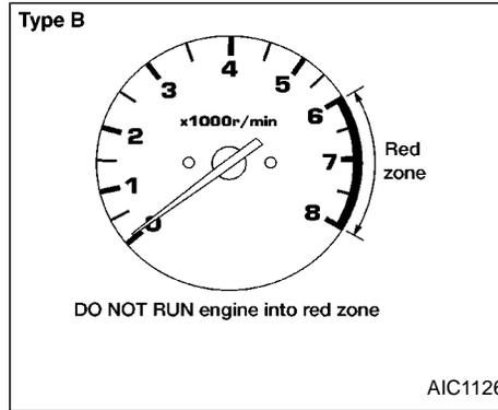
The tachometer indicates engine speed in revolutions per minute (r/min).
