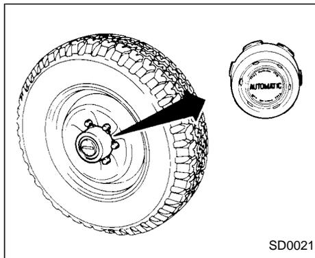
The auto-lock free-running hub is designed to allow for automatic four-wheel drive engagement when the shift lever is moved to the 4H or 4L position. If your vehicle is equipped with this system, follow these operational cautions:
