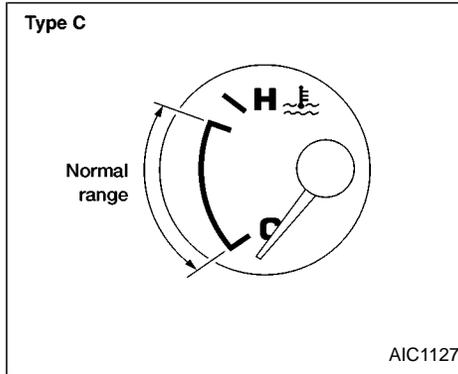
The gauge indicates the engine coolant temperature.
