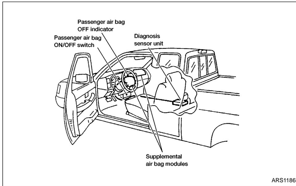
The driver supplemental air bag is located in the center of the steering wheel. The passenger supplemental air bag is located in the top right section of the instrument panel.
