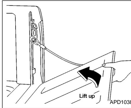
To open the tailgate to the lowest position, lift the tailgate to a 45 degree angle, then release the support cables.
