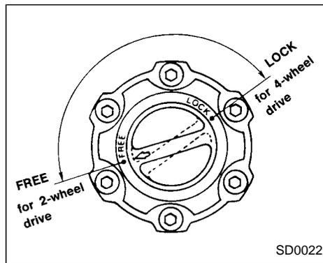
The manual-lock free-running hubs are designed to allow you to engage or disengage the front drive shaft to the front wheels. Before driving, set the free-running hub to the desired position:
