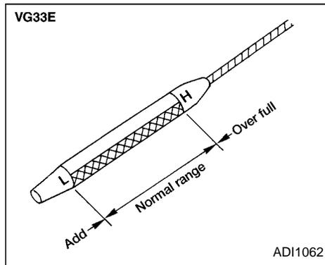
5. Remove the dipstick again and check the oil level. It should be between the H (High) and L (Low) marks. If the oil level is below the L (Low) mark, remove the oil filler cap and pour recommended oil through the opening. **Do not overfill.**
