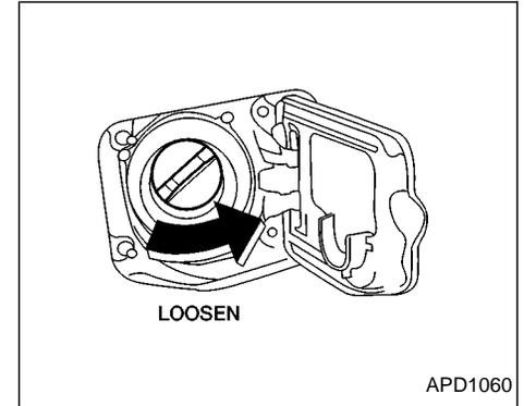
The fuel filler cap is a screw-on ratcheting type. Turn the cap counter clockwise to remove. Tighten the cap clockwise until ratcheting clicks are heard.
