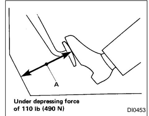
With the engine running, check distance A between the upper surface of the pedal and the metal floor.
