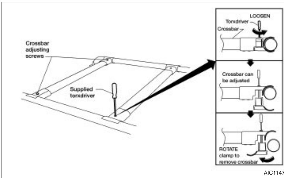
The front and rear crossbars can be adjusted forward, backward, or be removed. Use the torxdriver located in the tool kit to loosen both crossbar adjusting screws. Position the crossbar as needed and then tighten the crossbar adjusting screws. Place
