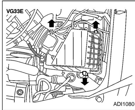
The filter element should not be cleaned and reused as it is given a special treatment. We recommend it be replaced according to the maintenance intervals shown in the "Maintenance" section of this manual. When replacing the filter, wipe the inside of the air cleaner housing and the cover with a damp cloth.
