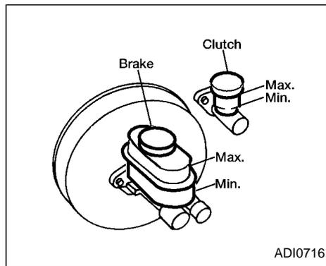
Check the brake fluid level in the reservoir. If the fluid level is below the MIN line or the brake warning light comes on, add **DOT 3** fluid up to the MAX line.
