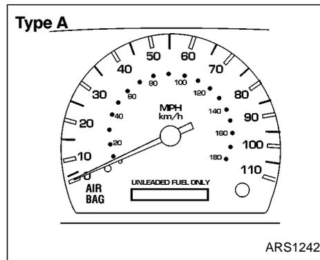
The supplemental air bag warning light, displaying **AIR BAG** in the instrument panel, monitors the circuits of the supplemental air bag system. The circuits monitored by the supplemental air bag warning light are the diagnosis sensor unit, the supplemental air bag modules and all related wiring.
